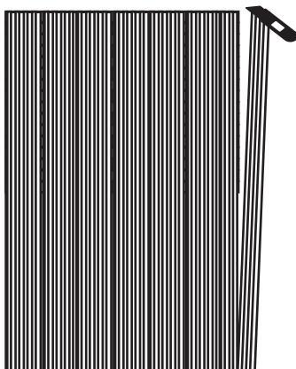
9. Cut off any excess panels at the edge of the application area, using a jigsaw or bladed knife, before fixing the last one.
