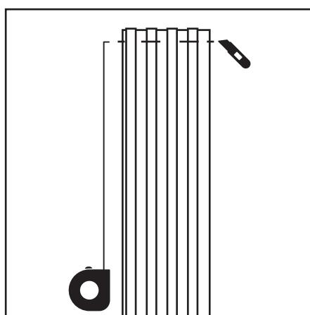
2. Cut the panels to the above mentioned/ measured size using a jigsaw or bladed knife.
